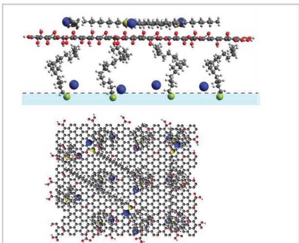
Schematic representation of organic monolayer coupled with a graphene plane
